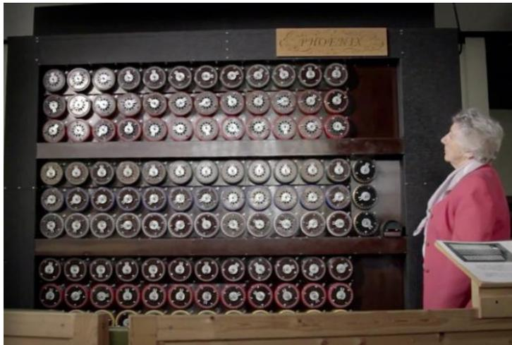
communications during World War II, the British Bombe is conceived of by computer pioneer Alan Turing and Harold Keen of the British Tabulating Machine Company. Hundreds of bombses were built, their purpose to ascertain the daily rotor start positions of Enigma cipher machines, which in turn allowed the Allies to decrypt German messages.
