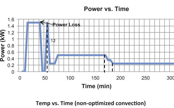
In comparison to convective heating, radiant heating achieves decontamination temperatures faster, with less power input, and without air movement
