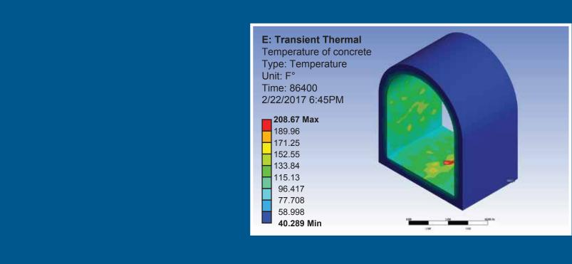
Simulation results show operation-scale heating can be achieved with similar hardware and extended heating times
